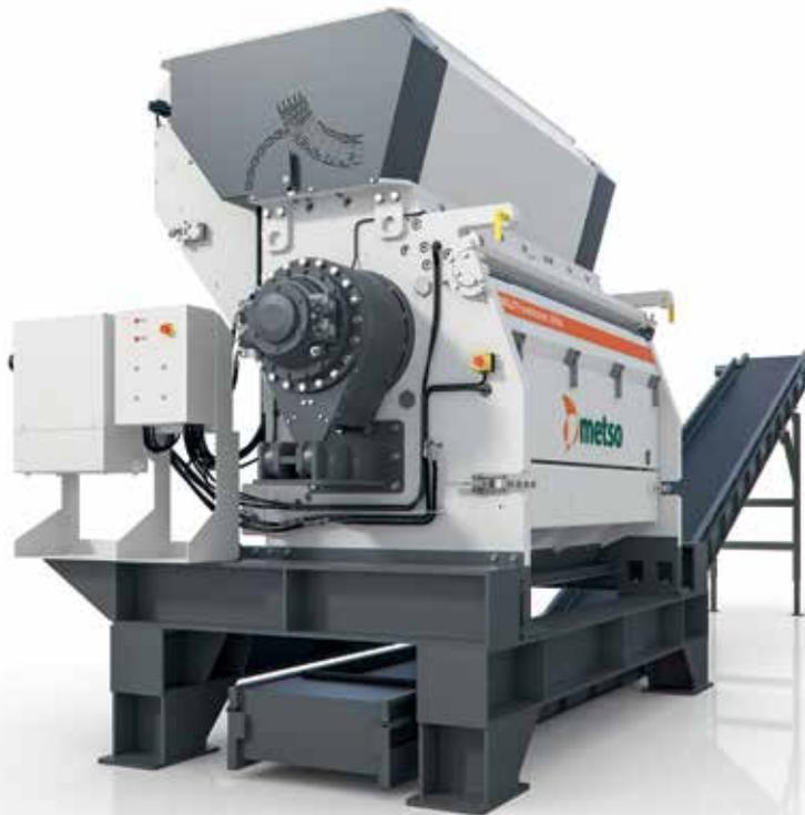
The M&J FineShred series consists of one-shaft shredders ideal for all recycling purposes. The shredder handles a wide range of different materials in bales, rolls, bricks or loose – and is highly suitable for RDF production.
